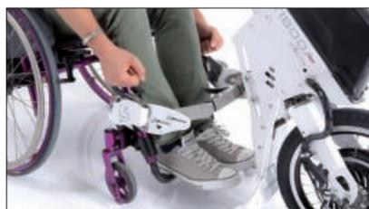
Put the safety levers of Tiboda® down (F)
