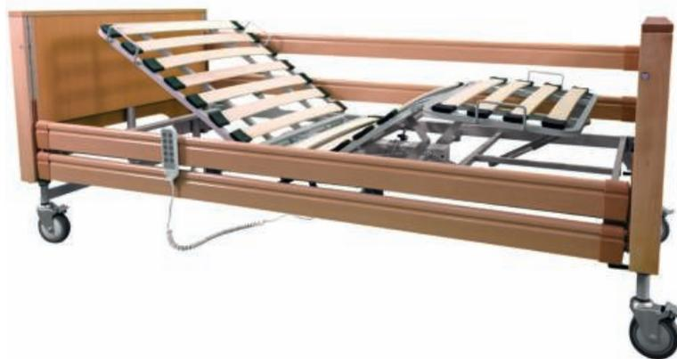
Steel tubular frame, powder coated. 4 swivel casters 125mm Ø with brakes. Head and footboard in wood, aluminium bedrails, wooden effect. Patient lift and IV pole supports. Compliant to UNI CEI EN 60601-2-52 for medical beds.
