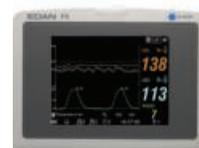
Light weight and compact. Closable LCD display 5.6". Basic functions: FHR, TOCO, DECG, IUP and automatic recognition of fetal movement. Signals overlap verification to differentiate twins FHR (ONLY FOR Ltd566). With printer, 12-hour memory, software for PC and USB port.
